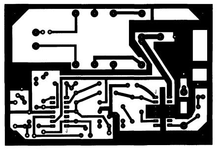
fig. 7. Full-size printed-circuit layout for the tunable audio filter. Drilled PC boards are available (see footnote below).
